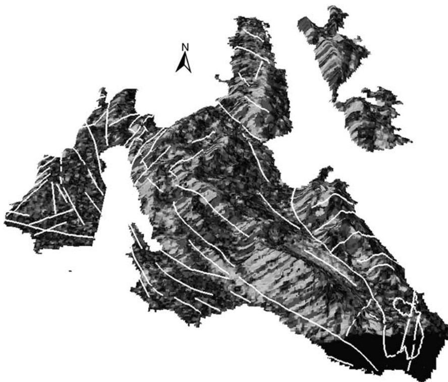
Fig. 5. Three-dimensional representation of the interferogram obtained by processing a couple of ERS-1 and -2 SAR images covering Kefallinia, with the main fault system of the island superimposed.
