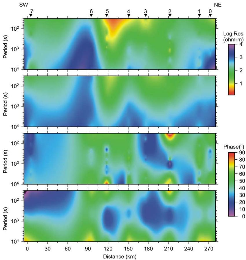
Fig. 7. The fit of the 2-D model responses to the observed data for the case of TE mode. From top to bottom: observed resistivity-model resistivity-observed phase-model phase.
