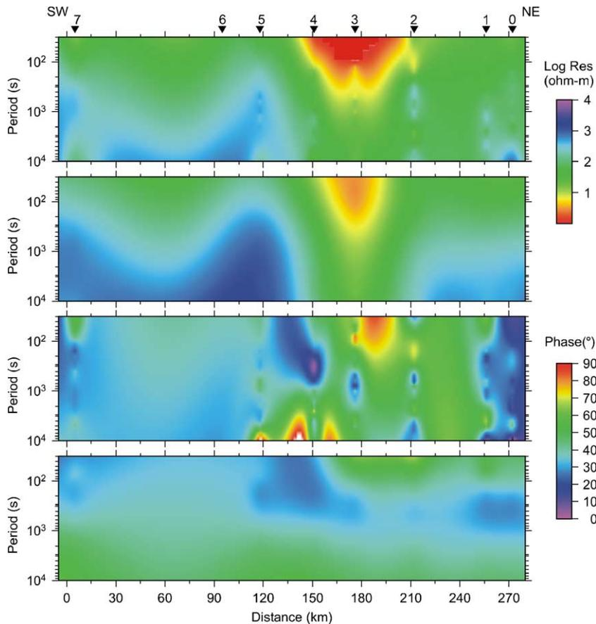
Fig. 8. The fit of the 2-D model responses to the observed data for the case of TM mode. From top to bottom: observed resistivity-model resistivity-observed phase-model phase.
