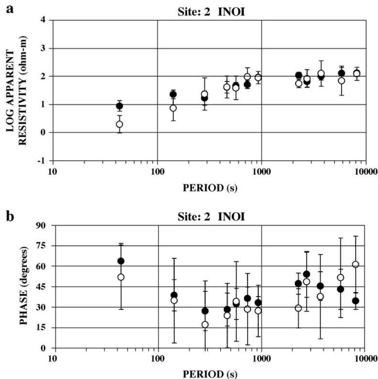
Fig. 2. The LMT data for site 2. (a) Period variation of apparent resistivity values in the measured directions. (b) Period variation of phase values in the measured directions. Solid circles: north–south direction; open circles: east–west direction.
