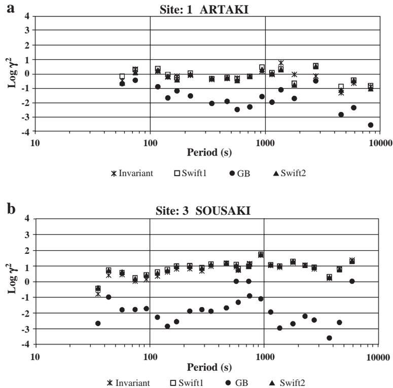
Fig. 3. Period variations of the  $\log \gamma^2$  misfit criterion for: (a) LMT site 1. (b) LMT site 3. Stars: 1-D model; open squares:  $5N$  free parameter 2-D model; solid circles:  $4N+1$  parameter 2-D model; solid triangles:  $7N$  free parameter 2-D model.
