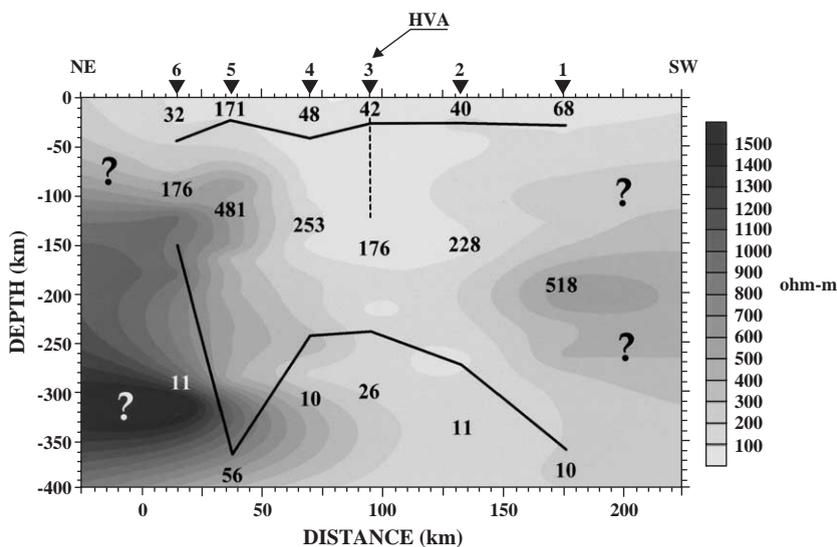
Fig. 5. The collated “Most Squares” 1-D models superimposed on a contour section based on the Niblett–Bostick transformation. Solid lines and figures: “Most Squares” layer boundaries and resistivities in  $\Omega\text{-m}$ ; scale bar: Niblett–Bostick resistivity range; question marks: poorly resolved structures.
