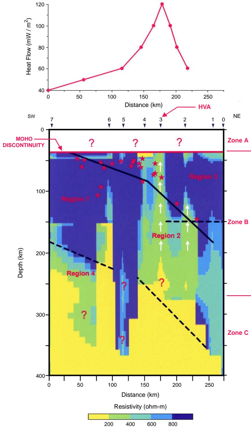
Fig. 6. The 2-D model together with seismic and heat flow data. Red solid stars: earthquake loci by Hatzfeld et al. (1989); black solid lines: Wadati-Benioff zone by Papazachos et al. (2000); dashed lines: inferred electrical boundaries; white arrows: probable magma flow; question marks: poorly resolved structures.
